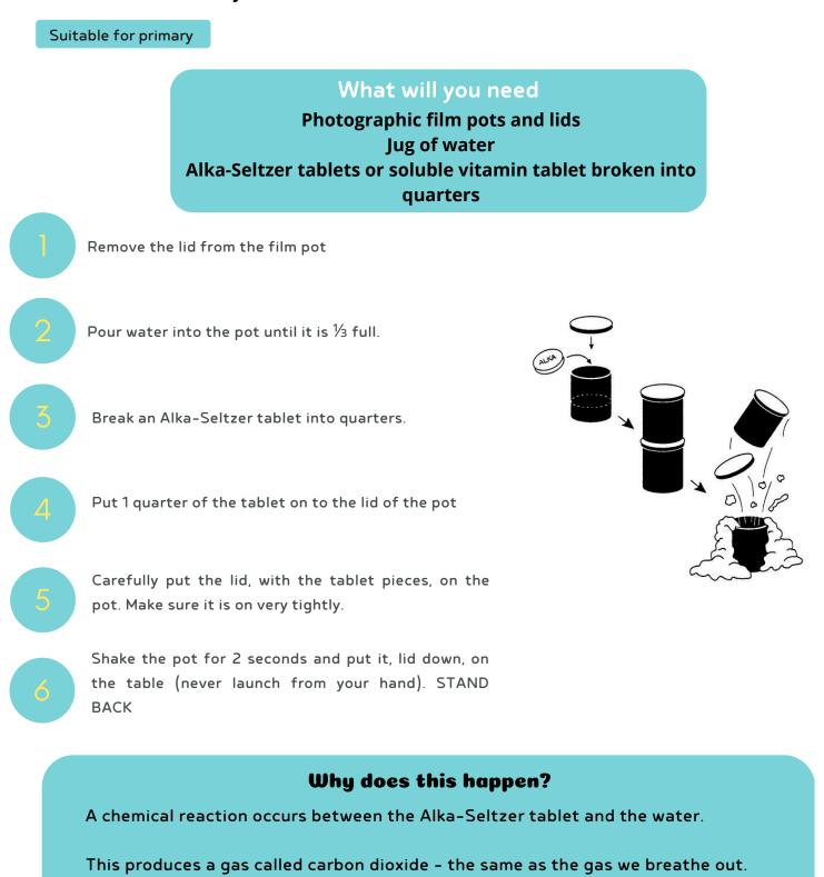
The gas builds up inside the film pot, increasing the pressure, until the lid is forced off.
